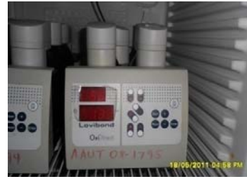
Digital BOD incubator, Lovibond BOD system oxidirect.
