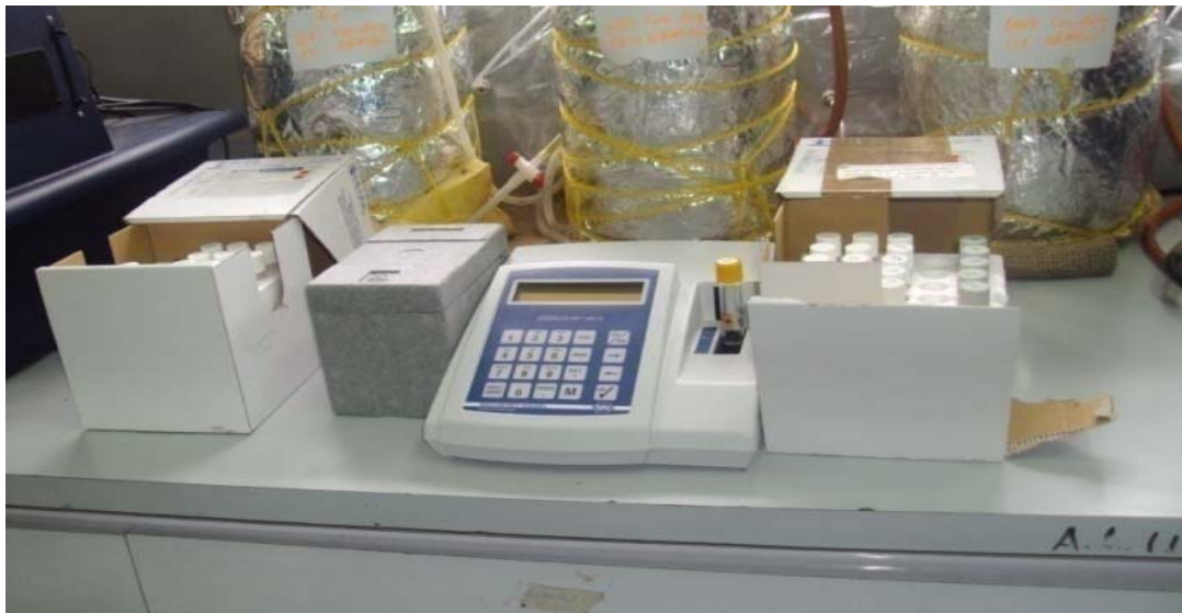
Measurements of the COD value of the different mix of substrate using NANOCOLOR multiple parameters.
