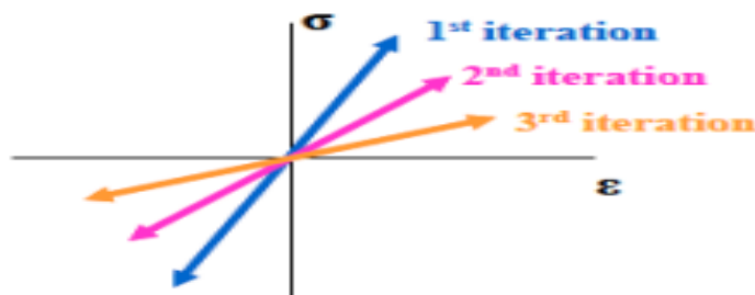
Figure 3-22: G changes with each iteration of the earthquake.
