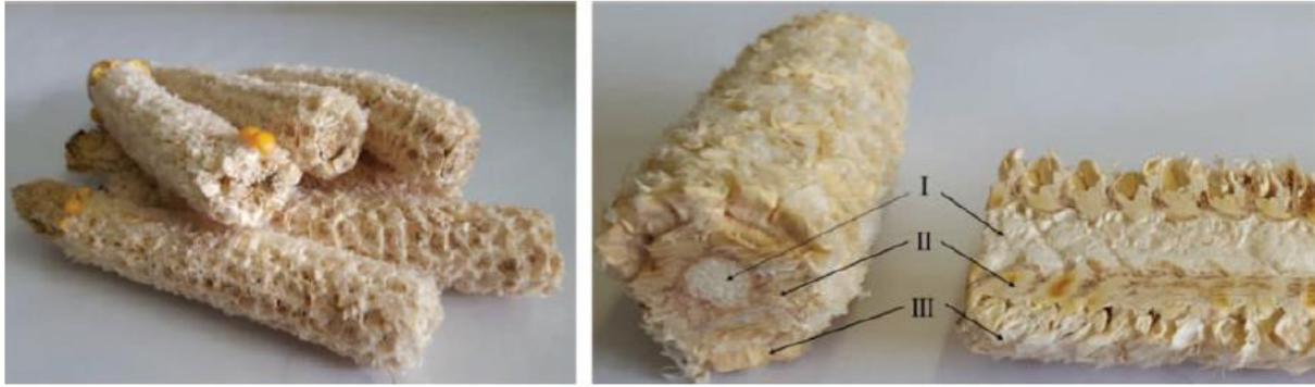
Fig 2.2 Corncob macrostructure: a) general view and b) longitudinal section (Jorge et al., 2016).
