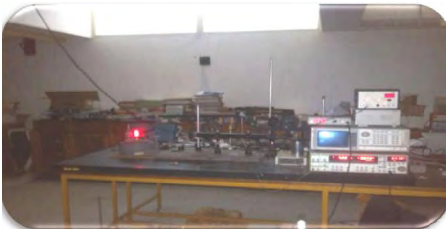
Figure 3.3.1.2: Photograph of experimental set up used for scattering intensity measurement
