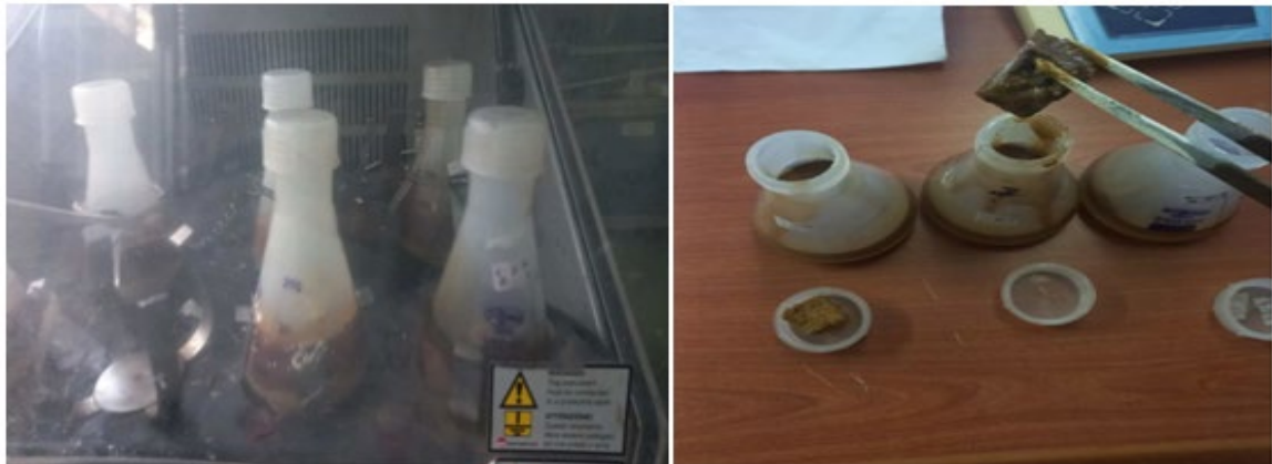
Placing the prepared oil/water/sorbent system on shaker Taking out the sorbent from flask
