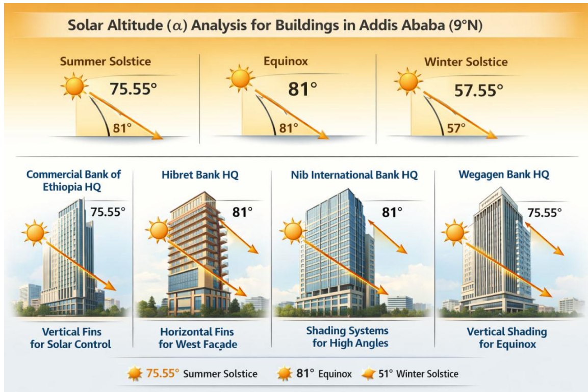
Figure 5.2: Solar Altitude ( \alpha ) and Sun-Breaker Performance at Addis Ababa's
