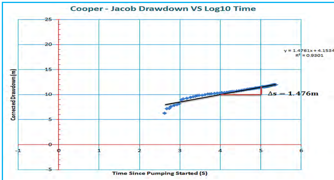
Figure A12. Copper-Jacob method for solution of non-equilibrium equation using the adjusted drawdown test data of MJBH-2. Drawdown is plotted as a function of time on semi-logarithmic paper.
