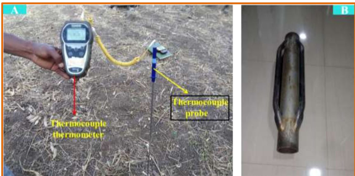
FIGURE 1.6: A. thermocouple probe and thermometer used for soil temperature measurements B. Custom-made sled hammer used to inject iron rod into 50 cm depth for temperature measurements (properties of RG Geothermal Ltd)
