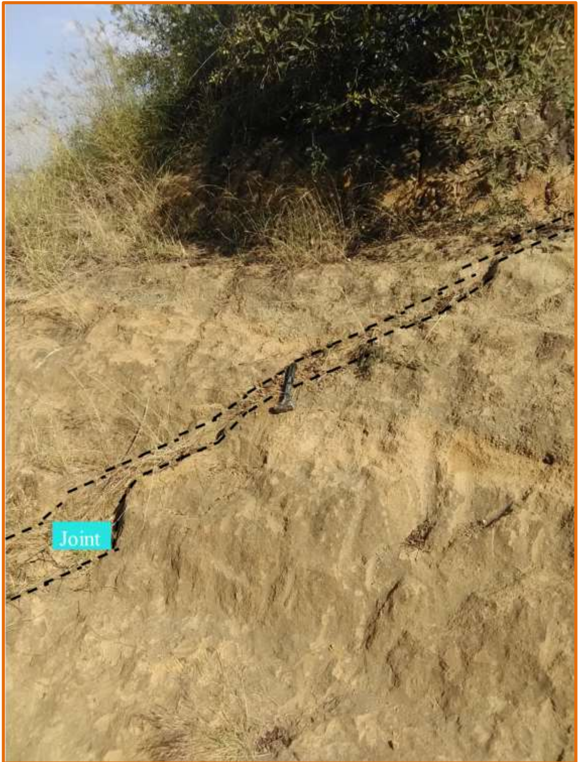
FIGURE 4.15: Exposure of lacustrine sediments that is located southeastern part of the study area.it is crossed by minor joint with spacing of 30 cm
