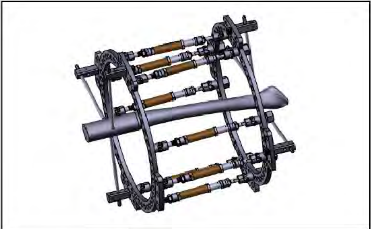
Figure 6.6 Ilizarov ring coupled with the proposed fixation device (designed using Solidworks).
