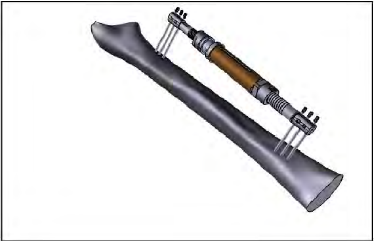
Figure 6.5 Unilateral fixation system (designed using Solidworks)
