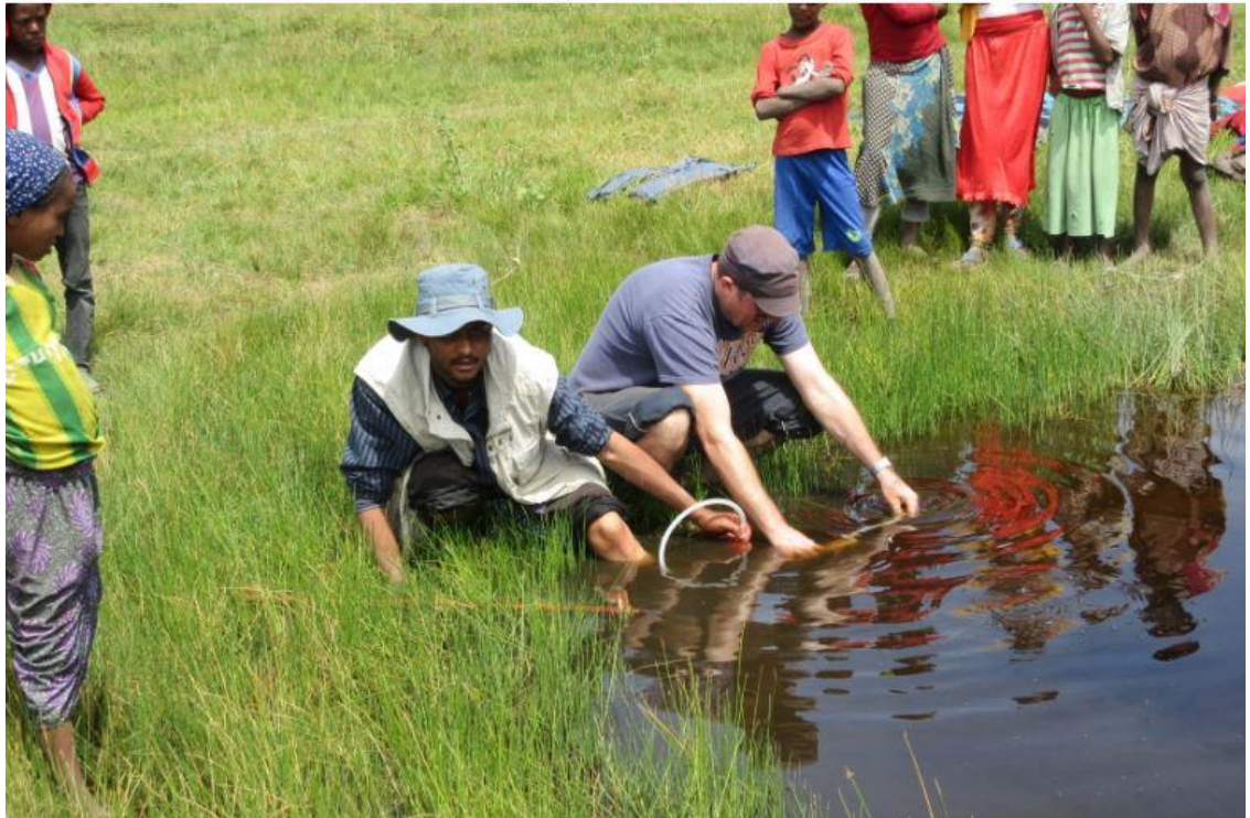
Figure 7. Gas sampling in the field at the top (flushing method) where prolonged flushing is conducted for approximately an hour and bottom (displacement method) where the funnel become submerged completely and the funnel will be inverted displacing water with gas bubbles
