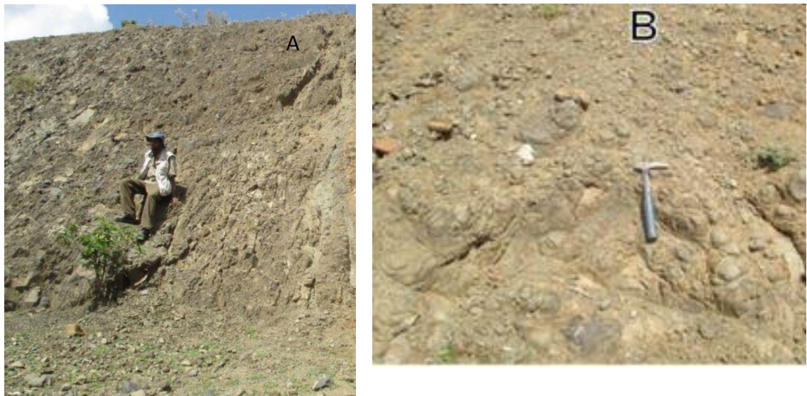
Figure 8. A. Pre rift basaltic formation from the western escarpment and B. exfoliation of highly weathered basalt from pre rift formation
