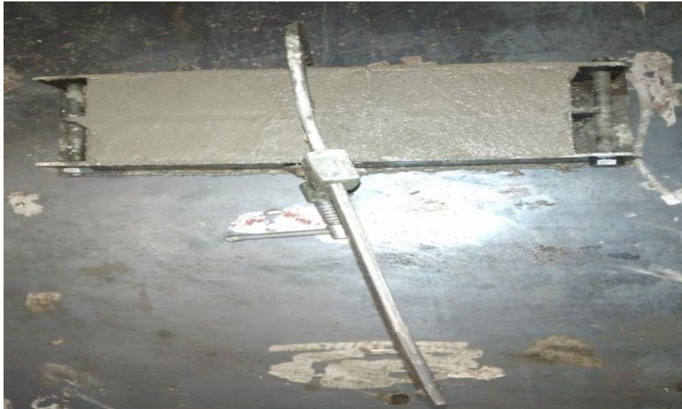
Figure 3.7— Mortar casted in to moulds
