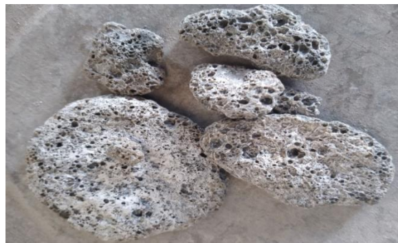
Figure 4.3 — Solid object formed during combustion of BTS samples at a temperature of 900°C
