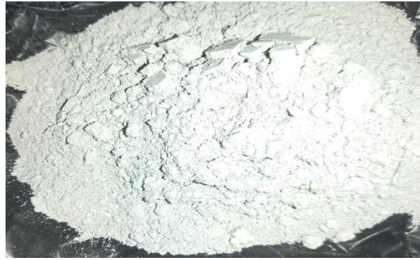
Figure 4.2 — BTSA sample after grinding of the ash for the combustion temperature of 750°C
