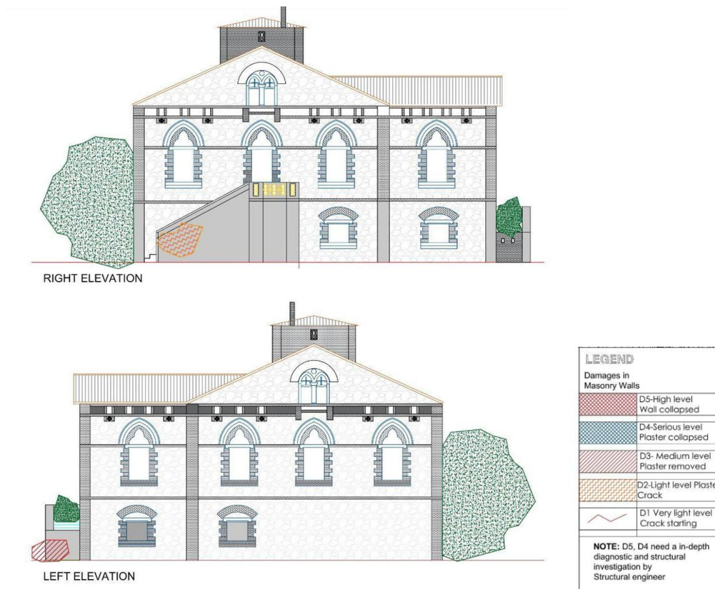
Figure 38. Elevation damage analysis 2
