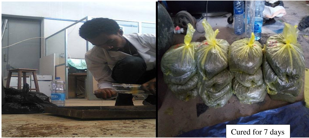
Figure 3-6 Samples preparation for a compaction test
