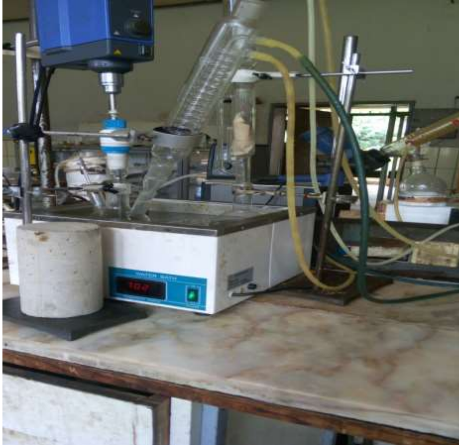
Figure 3.3: Experimental setups for extractive content determination
