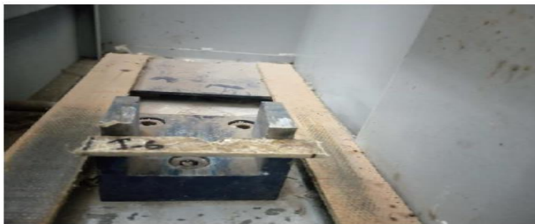
Figure 3.18. Impact strength test set up
