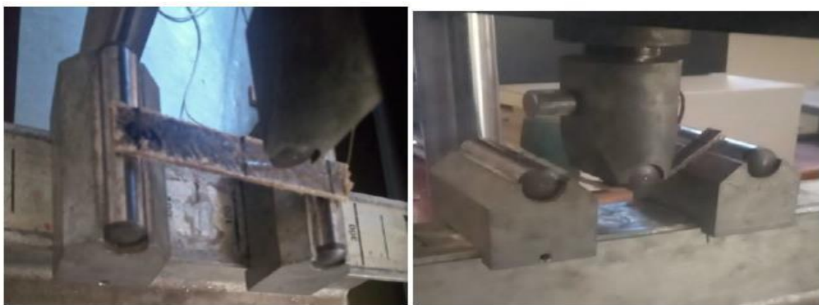
Figure 3.17. The composite specimen under flexural test examination.
