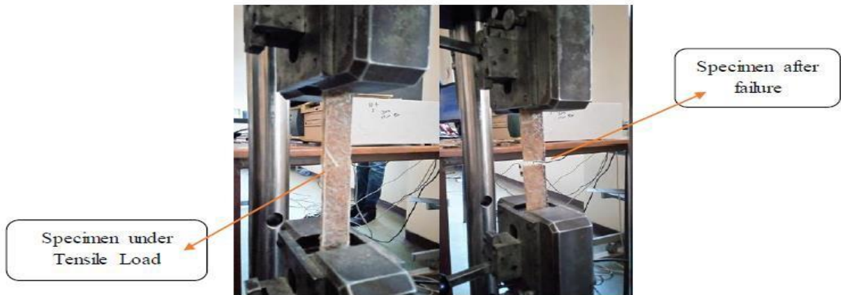
Figure 3.16. Tensile test specimens under examination
