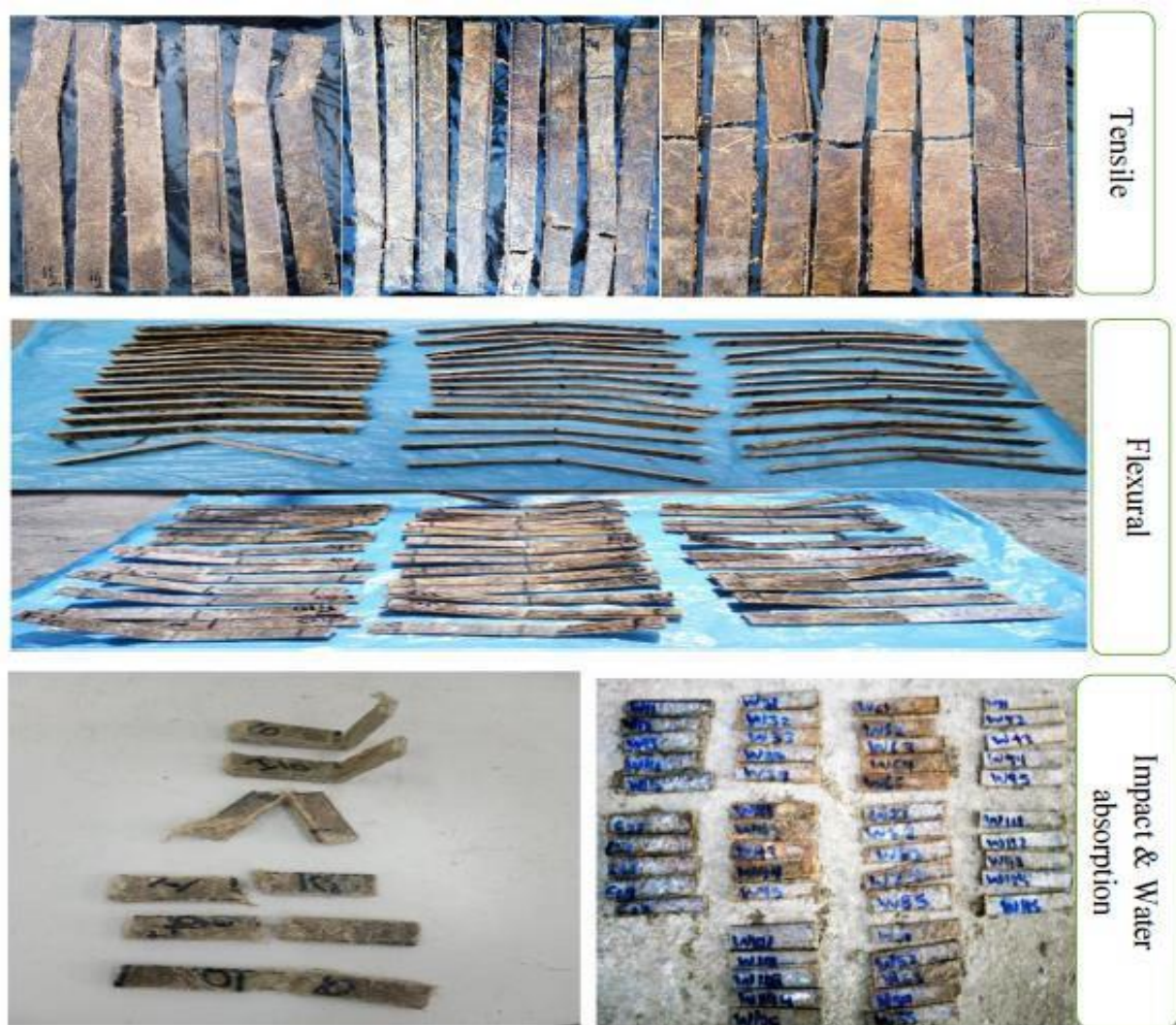
Figure 4.25. Tensile, flexural, impact, and water absorption specimens after test
