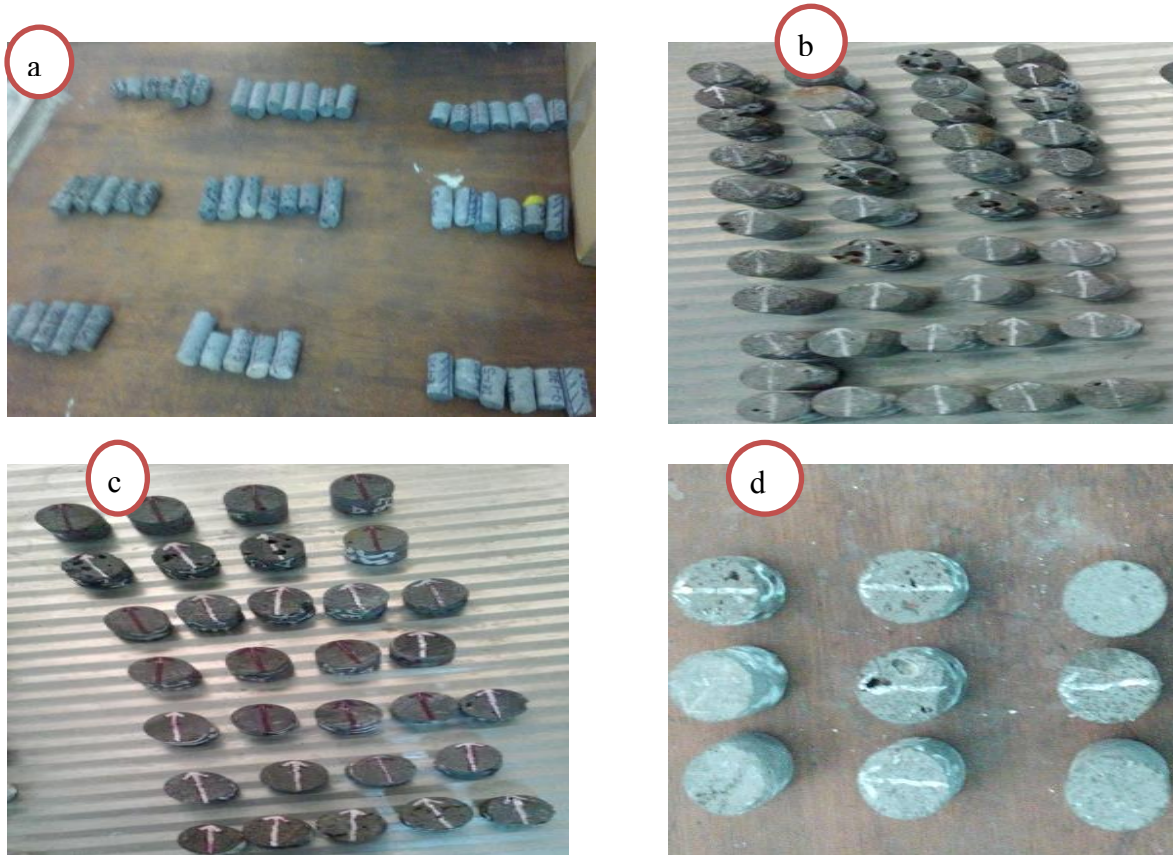
Plate 2.1.4B. prepared paleomagnetic samples in order to analyze paleomagnetism in laboratory. (a) Collected field paleomagnetic samples. (b) Prepared specimens for Thermal demagnetization. (c) Prepared specimens for Alternating field demagnetization. (d) Prepared specimens for mineralogy.
