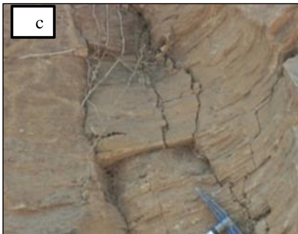
Plate 4.2.2.joint, (a, b) Columnar joints that exposed in basalt rock unit along road cut, (c) Joint intersection in Serdo area. Joints in the outcrop reveal a pattern which the traces of joints intersect and termination in the pre-existing joints .The joint terminated by branching and dying out .
