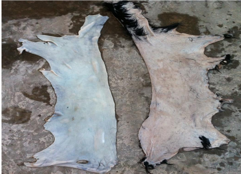
Fig. 4.15: Enzymatic method of unhairing and fiber opening (Left); conventional method of unhairing and fiber opening (Right).
