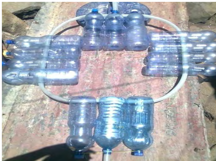
Figure 4.4: Batch mode operating scaled up SDWT system
