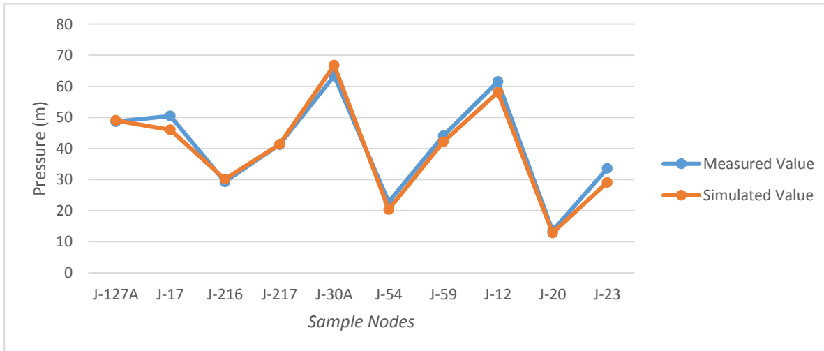
Figure 4.8: Graphical representation of simulated and measured pressure Value during low demand time
