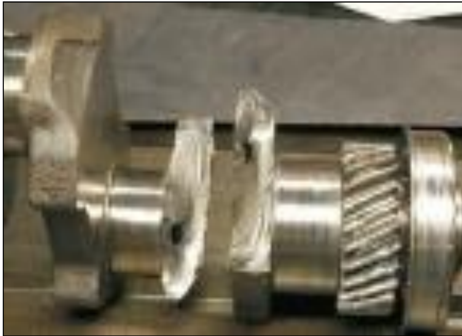
Figure 4: Example of fatigue failure
