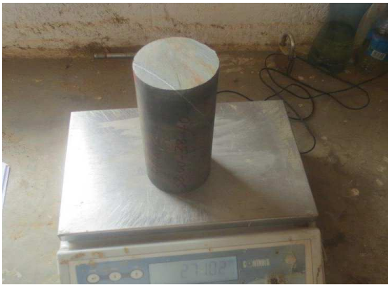
Figure 4.7. Core samples laboratory tests, weighing the core sample (left), UCS test of core sample (right)
