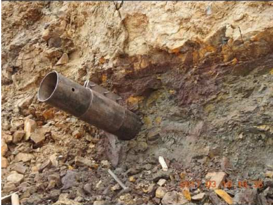
Figure 7.15. Sampling of infilling material from J2 joint set
