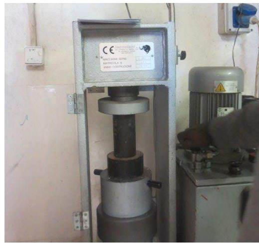
Figure 4.7. Core samples laboratory tests, weighing the core sample (left), UCS test of core sample (right)
