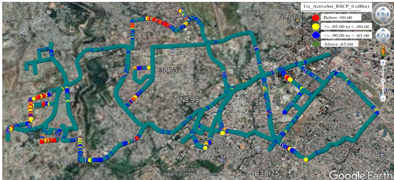
Figure 4.2 Data collection route and signal strength in the route
