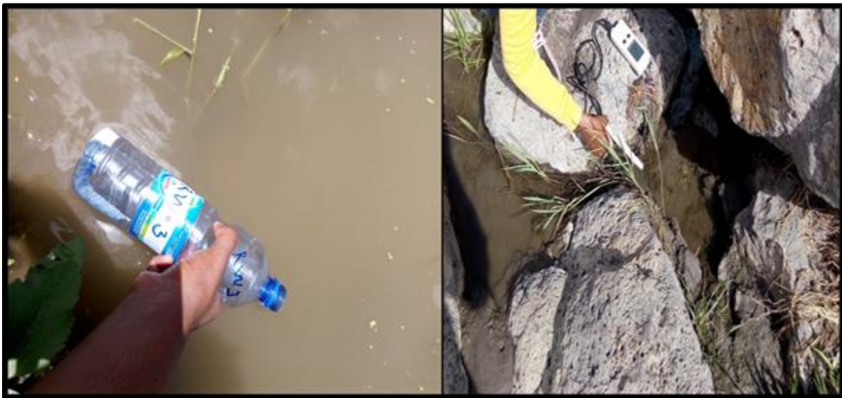
Figure 4.1. On field EC, pH measurement and surface water sampling.
