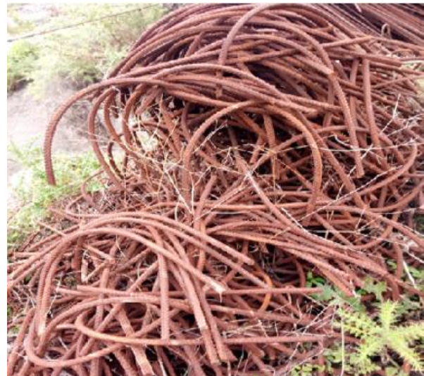
b) Reinforcement bars wastage
