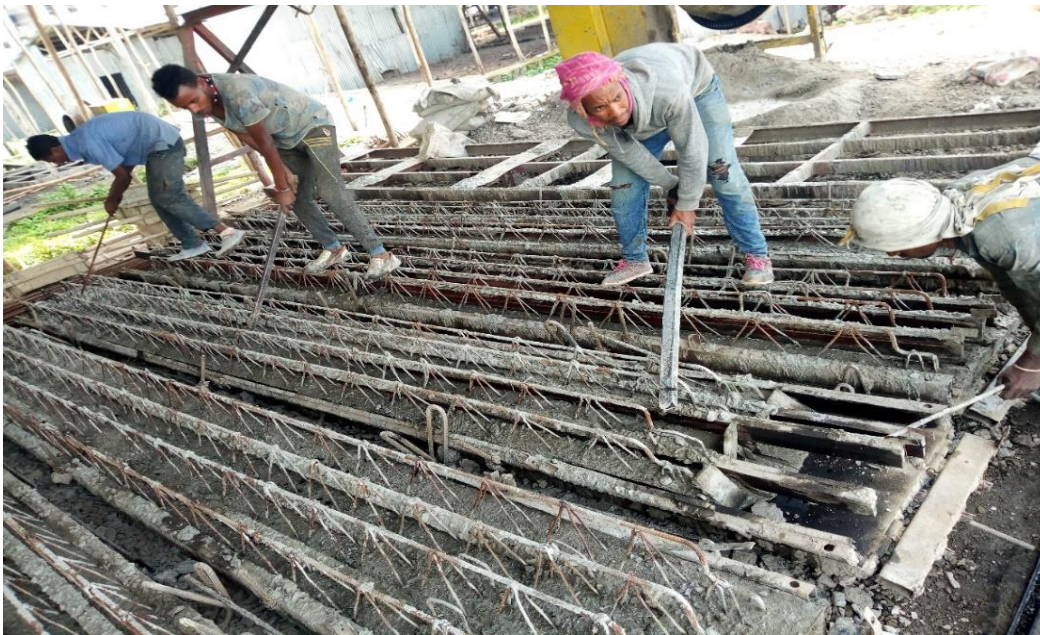
Figure 4.21 Mold dismantling practice on the production shades (picture taken by the researcher).
