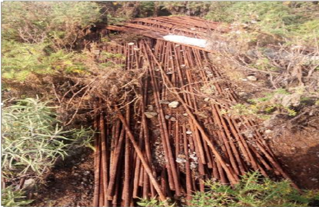
Figure 4.10 Reinforcement bar storage practice on the manufacturing shade through MSEs (picture taken by the researcher).
