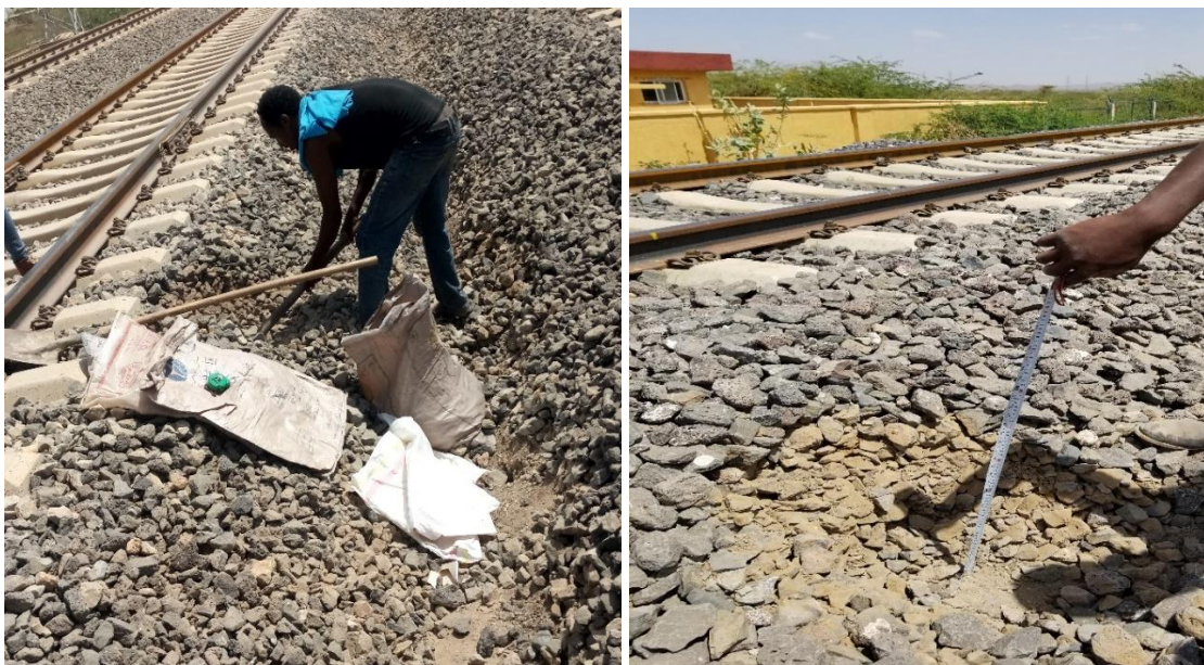
Figure 3.5 Extraction of Sample on the Left and Measuring of the Sampling Depth on the Right
