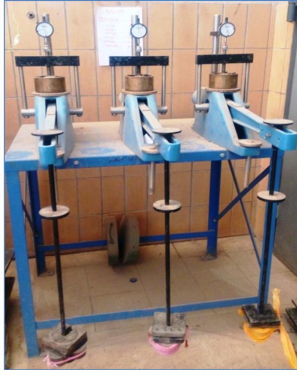
Figure 2.8 Table consolidation test apparatus
