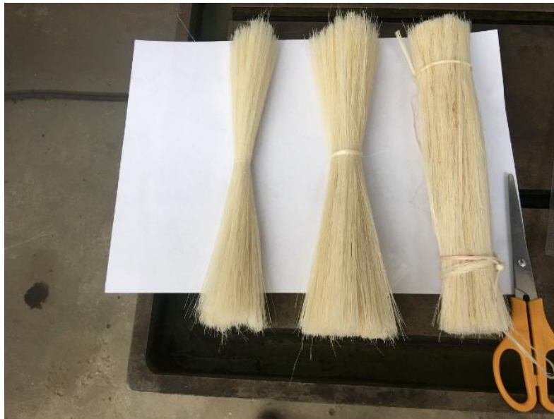
Figure 6 The Sisal fiber cut with the mold size
