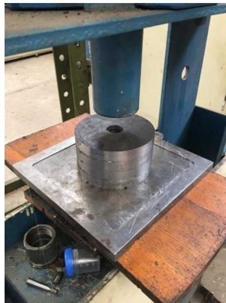
Figure 13 The sample inside the mold is being pressed by standard hydraulic press machine
