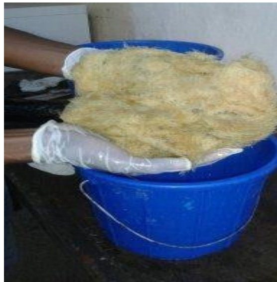
Figure 8 Pure Sisal fiber after mercerization
