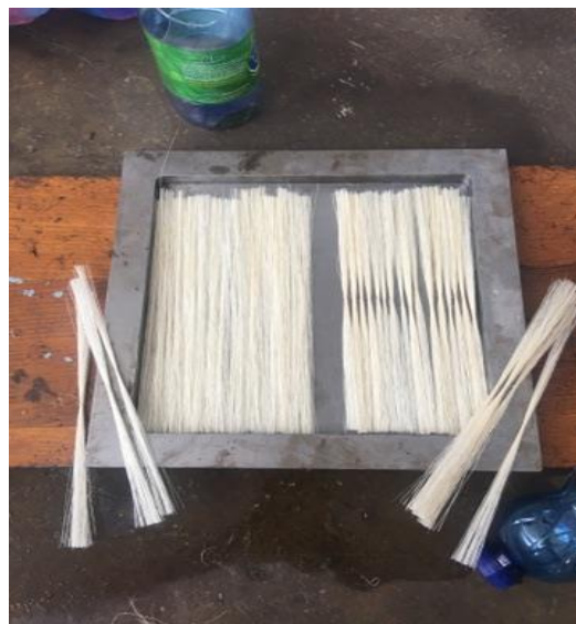
Figure 10 The mold, as fibers are being put on it for a trial production.
