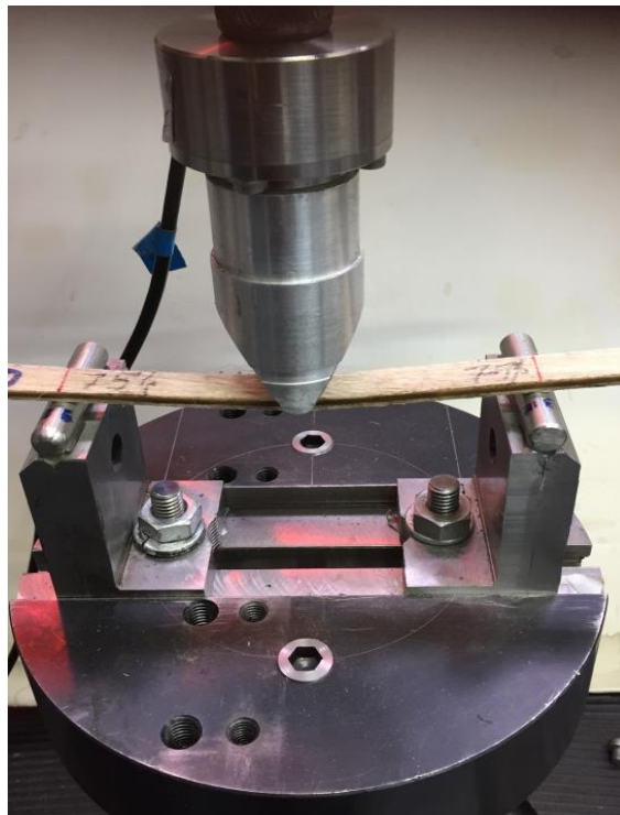
Figure 19 Fatigue / Static flexural test setup
