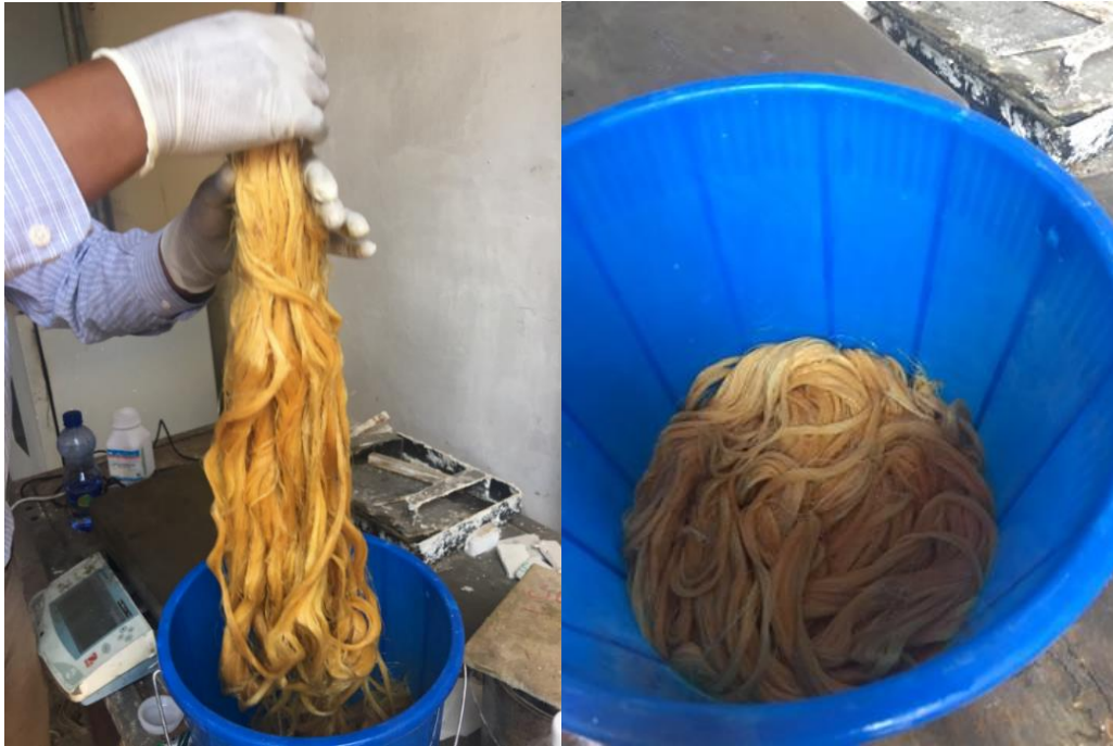
Figure 7 Sisal fiber soaked in NaOH solution for 24hrs
