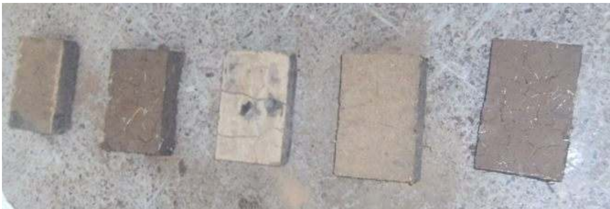
Fig.C.1 Stabilized earth blocks' photos
