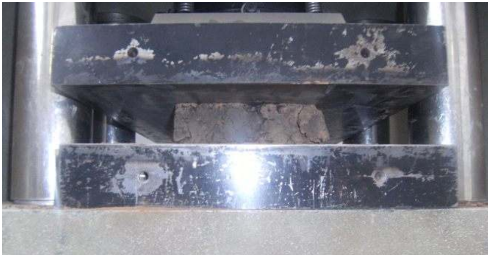
Fig.C.2 Compressive strength test and testing machine photos
