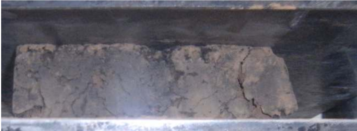
Fig .5.5 Large cracks in cement stabilized block (sample 5C) during compressive test
