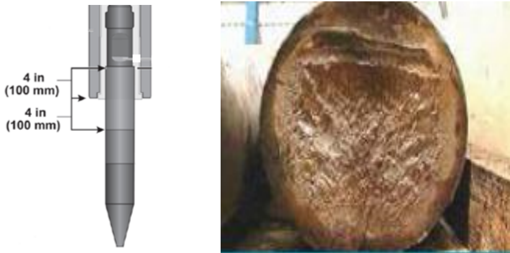
Fig.1.1.1. Fatigue fracture location & fracture surface on tool.
