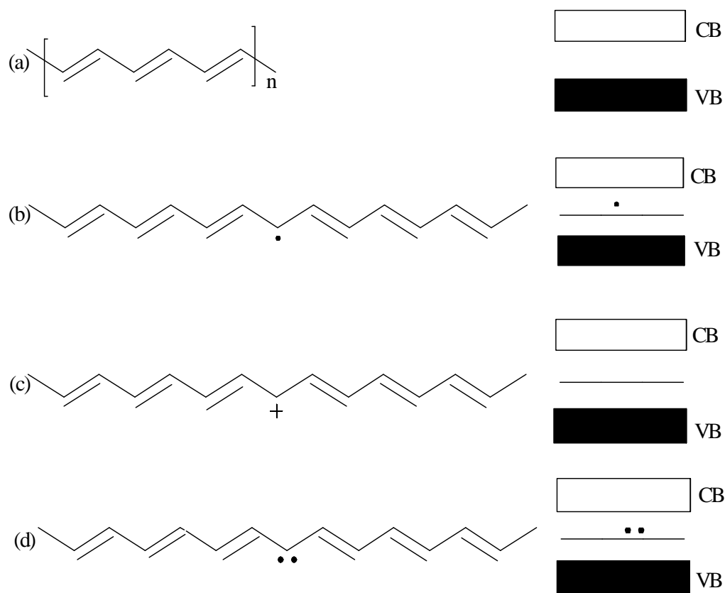
Figure 2.5: Left: Chemical structure of, (a) trans-polyacetylene, (b) neutral soliton, (c) positive soliton, and (d) negative soliton. Right: The corresponding band structure.
