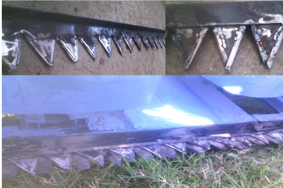
Figure 56 new modified cutter bar
