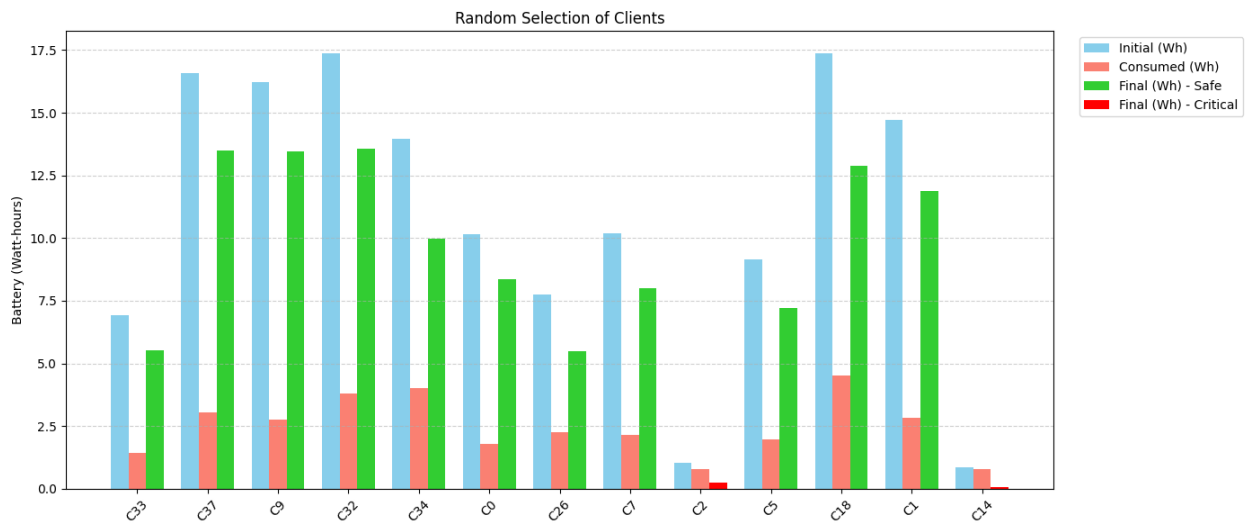
Figure 4.3: Random selection of clients and battery consumption illustrated resulting client dropout due to battery draining in a single communication round.
