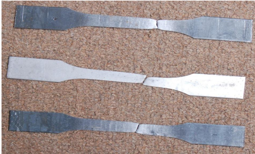
Figure 43 Sample test result for the three materials at the same strain rate.
