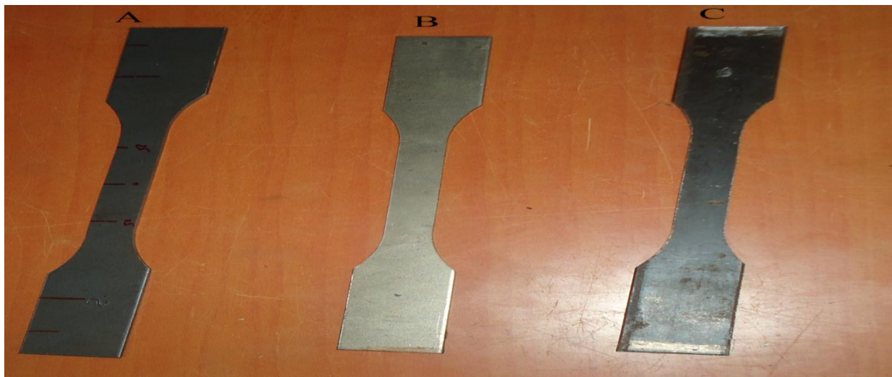
Figure 17 shows the specimens “dog bone” used for tensile testing
