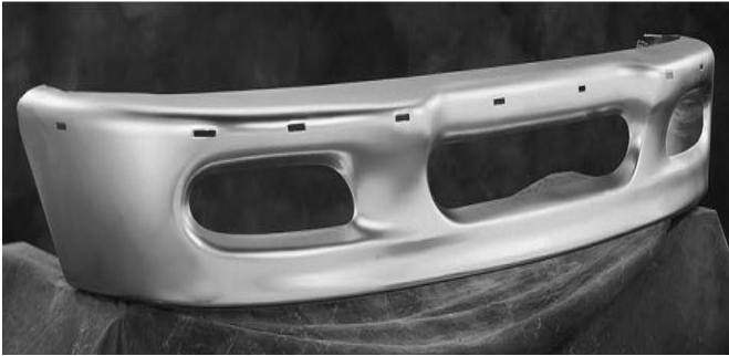
Figure 14 b) ford f150 pickup 559mm (22 inches) depth of draw with 50x1f steel. Aerodynamic styling source: [2]
