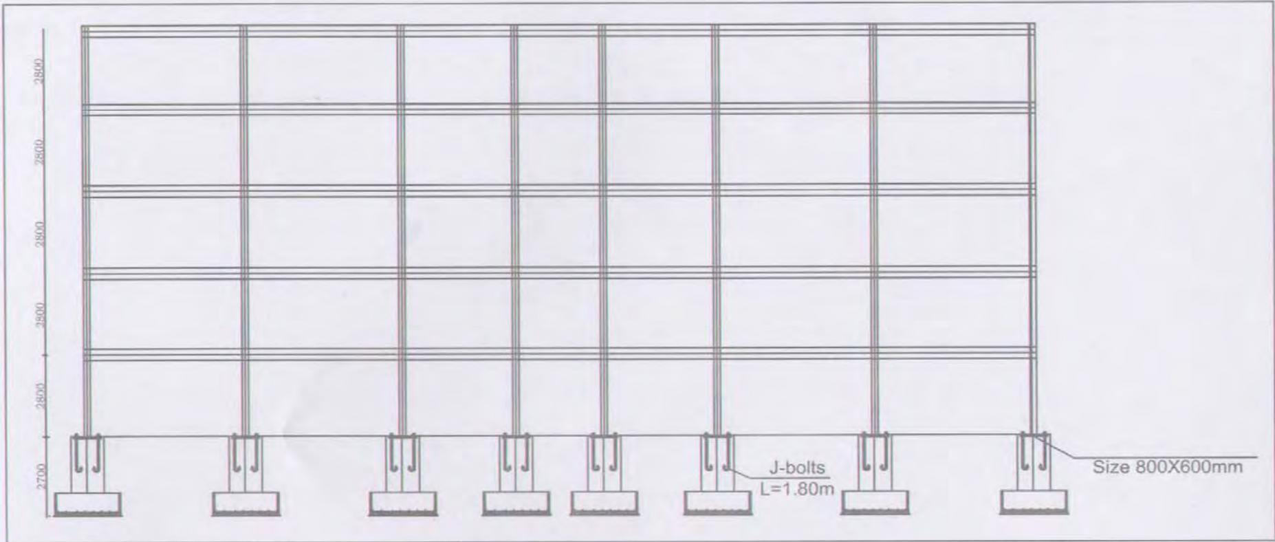
Fig. E-4 Frame on Axis 1-1 Sc1:50
