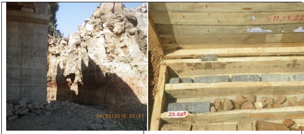
Plate 4.4 Weak zones/laterite/paleo soils/ underlain by basaltic rocks; creates stability differences, triggering factors for landslides hazard occurrence. Lithological log data obtained from coring activity tests drilled for bridge construction at Meshoalekia, Cherkos sub-city, Addis Ababa.
