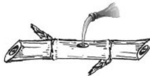
Figure E4 Pouring Solutions into culm
