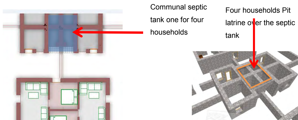
Figure 16: Communal septic tank
