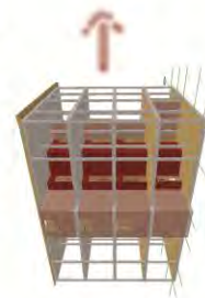
Initial core house (service +shellhouse) service at center to minimize the cost constructed by government
