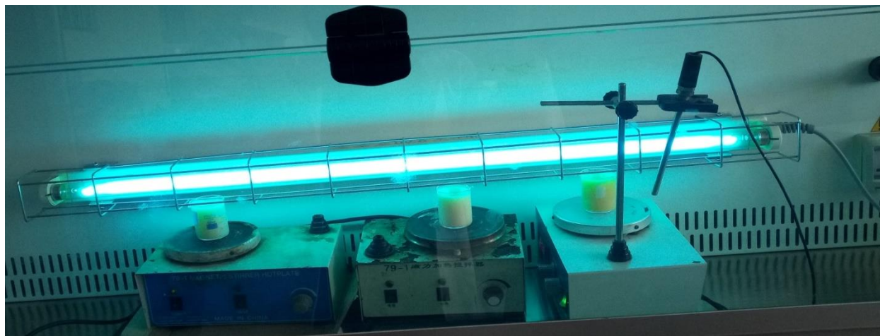
Figure 3.1. Photocatalytic experiment in a microbial hood
