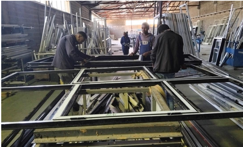
Figure 20. Glass stop (Ferma) cutting & installation
