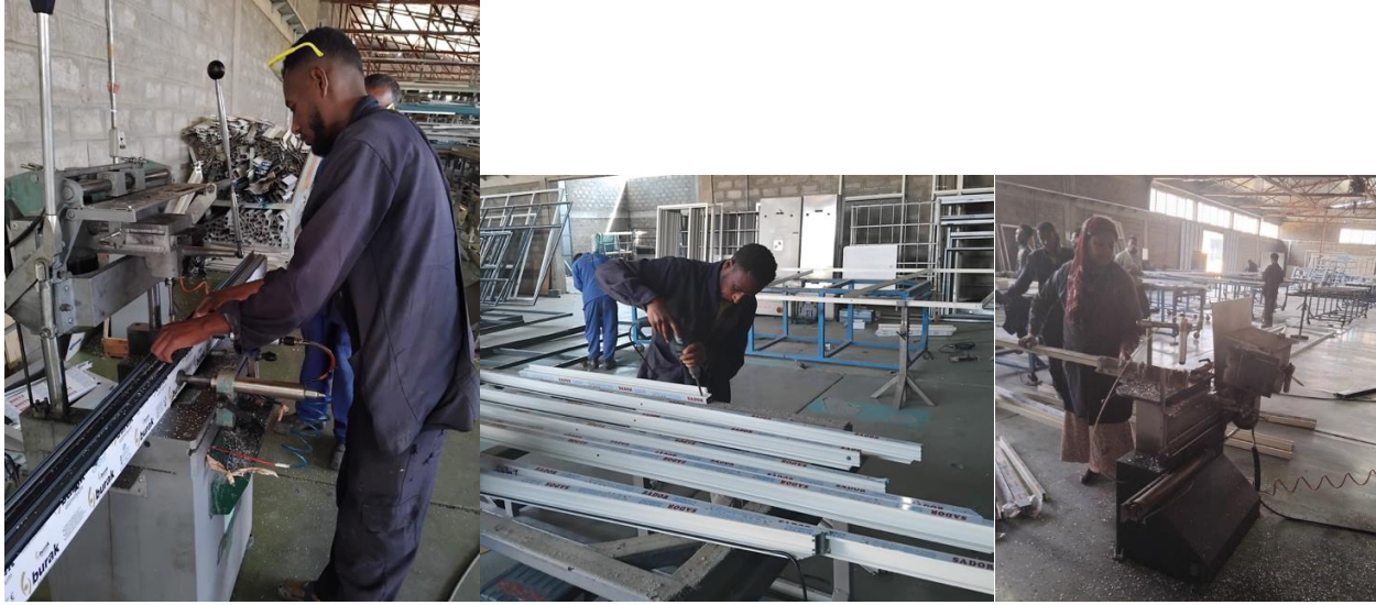
Figure 17. Routing, Drilling, and Milling
