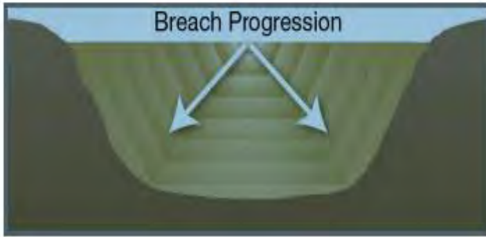
Figure 2-1 overtopping trapezoidal breach progression (FEMA, 2013)
