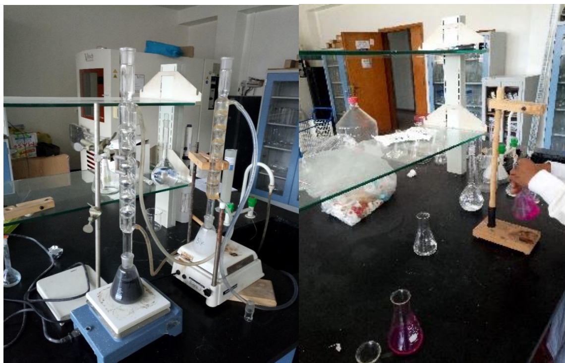
Figure 4.14 Modified Chapelle Test Experiment Under Investigation
