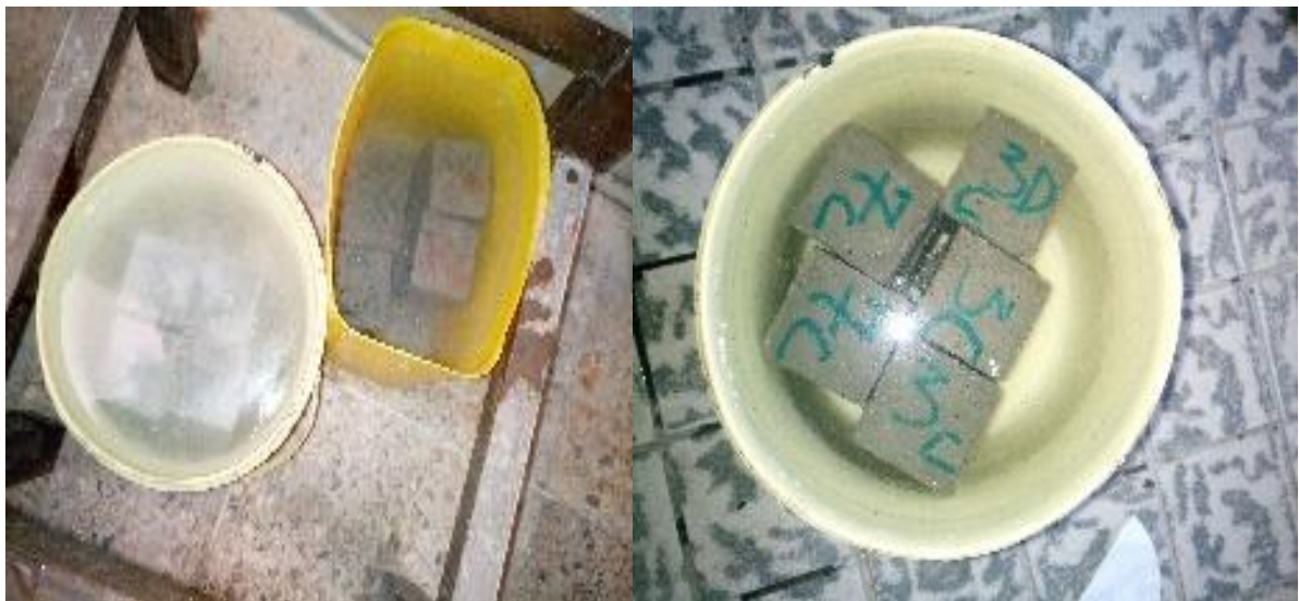
Figure A.E.8 Mortar Cube Curing Pond Used for the Study
