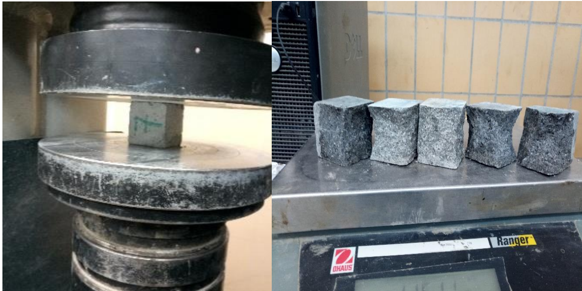
Figure A.E.7 Compressive Strength Test and Tested Cubes
