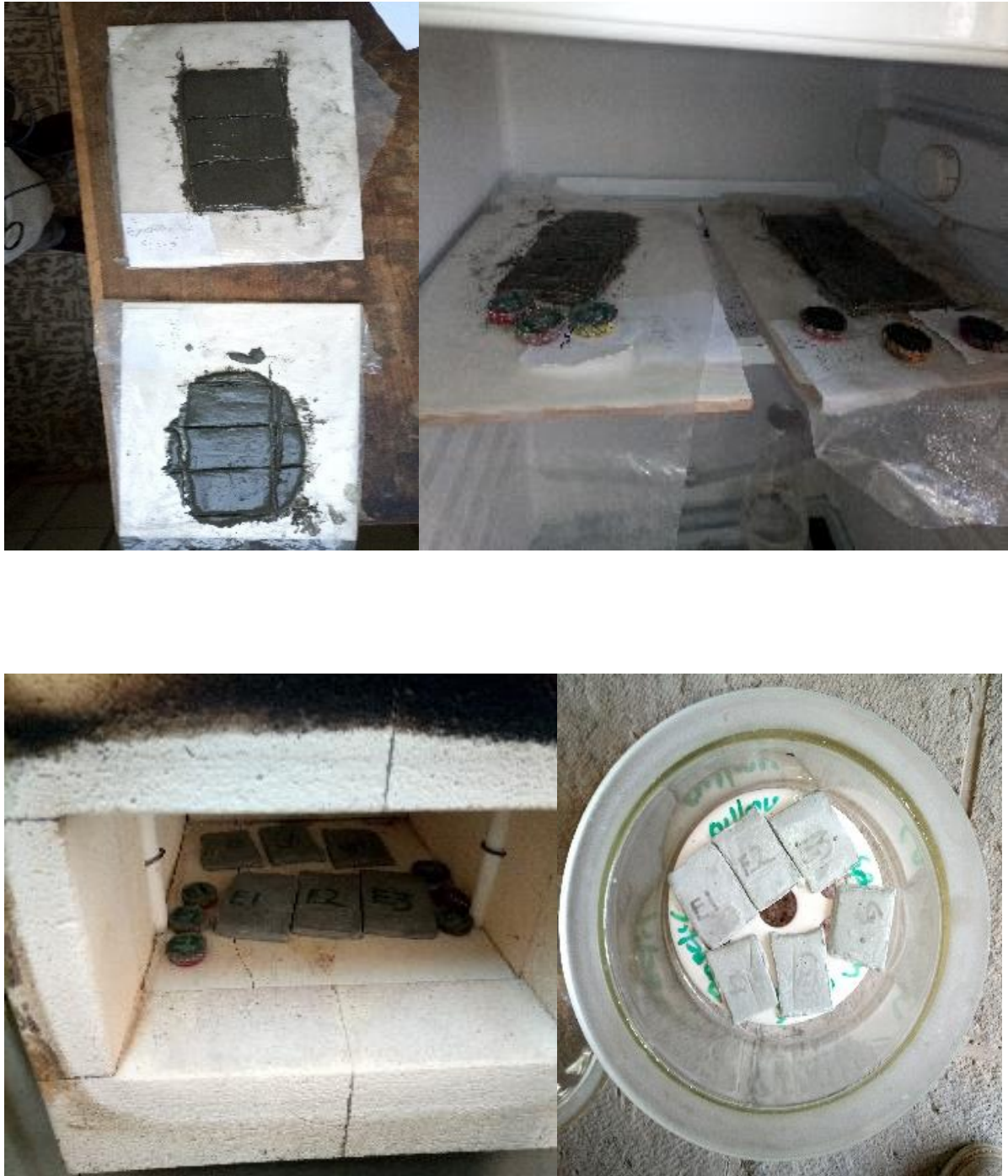
Figure A.E.4 Samples in the Process of Bound Water Determination
