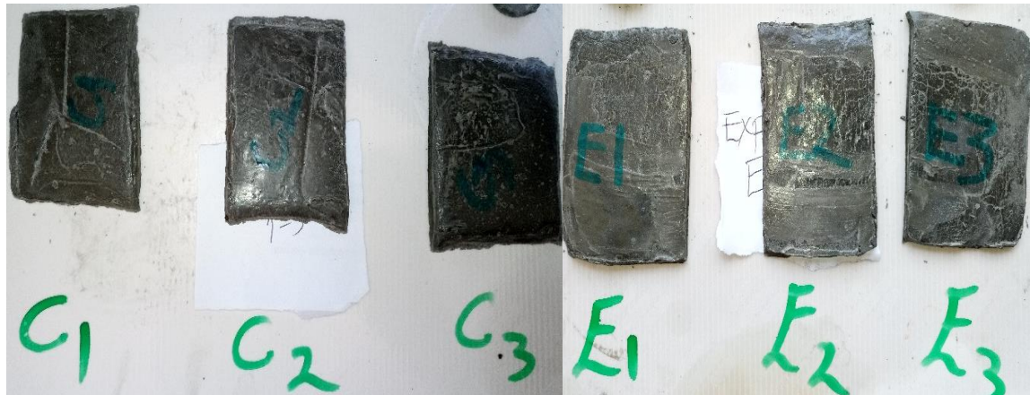
Figure 4.12 Samples Prepared for Bound Water Determination Test
