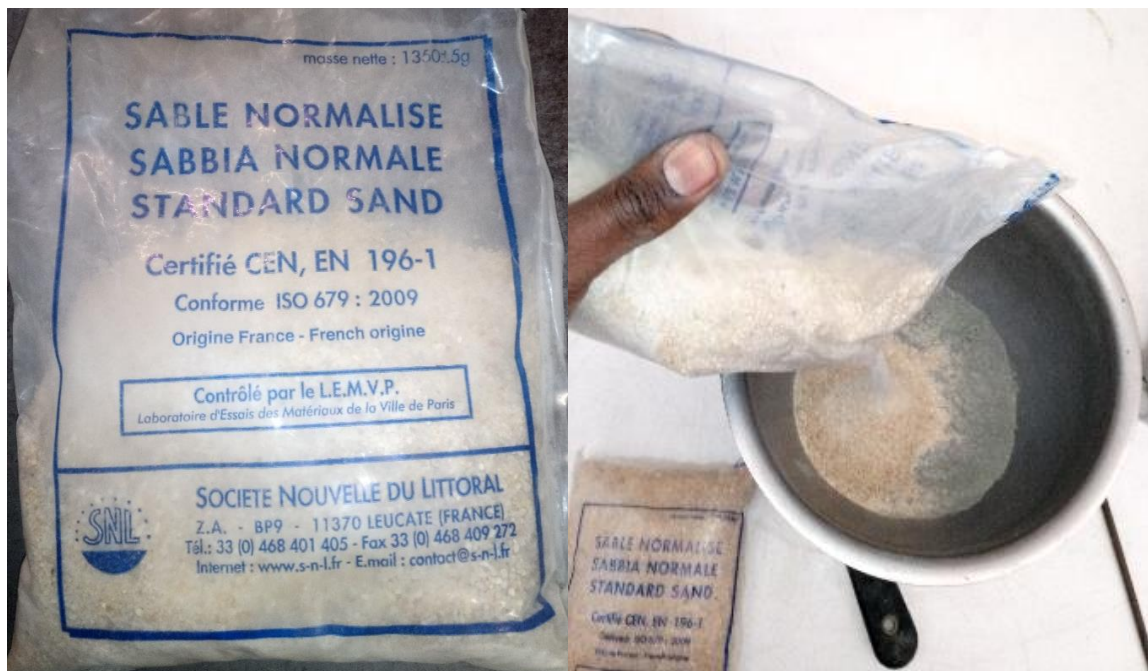
Figure 3.3 Standard Sand in Polyethylene Bag and During Pouring into Mixer (Right)
