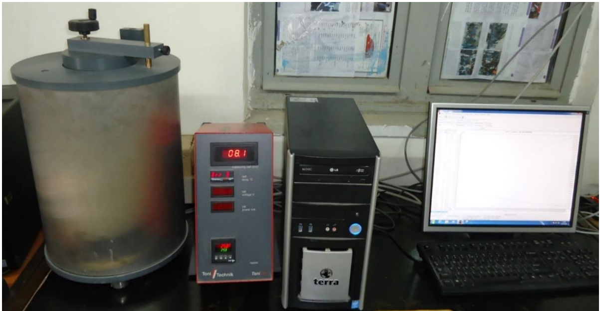
Figure 4.5 Heat of Hydration Measuring Calorimeter
