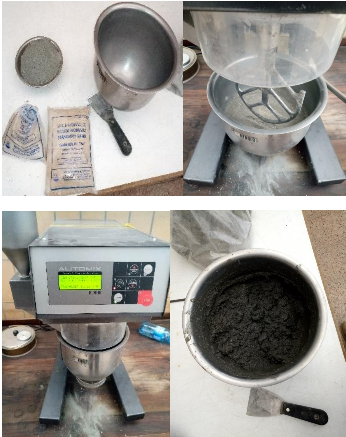
Figure A.E.6 Materials, Automatic Mixer and Mixed Paste
