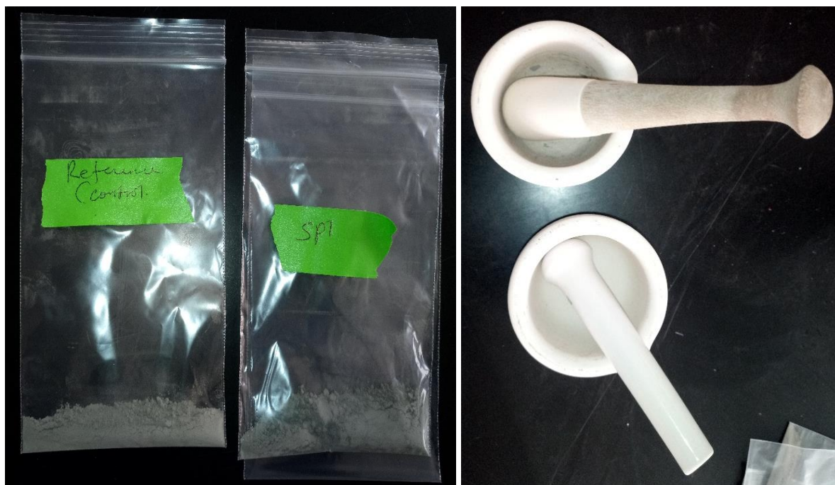
Figure A.E.3 Samples for XRD and Crushing Agate
