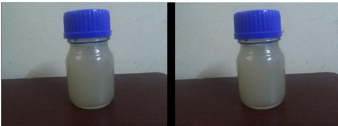
Figure 5: The nanocellulose suspension obtained from sugarcane bagasse after pretreatment and hydrolysis process
