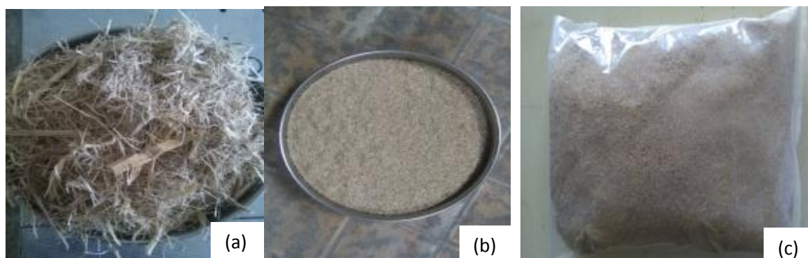
Figure 4: Sugarcane bagasse sample (a) as received from Fincha Sugar Factory (b) the grounded bagasse using laboratory mill (c) grounded bagasse was packed in polybags
