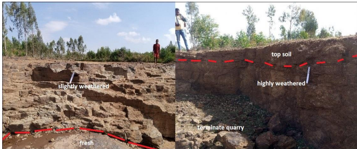
Figure 2.3: Ignimbrite unit is exposed in the east part of the study area near the Hamassa river (terminated Quarry site).
