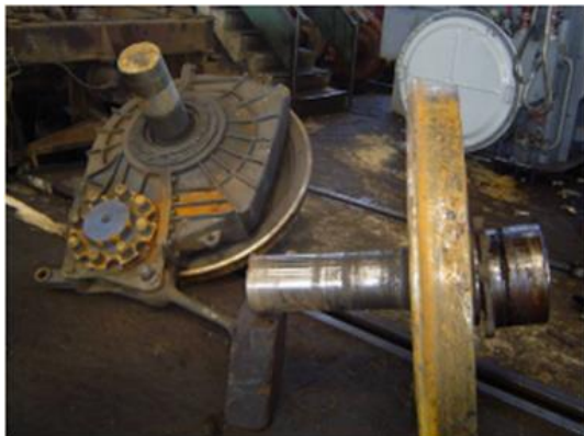
Figure 2.3: Fracture of the traction shaft in section 3 (Fig.2.1)
