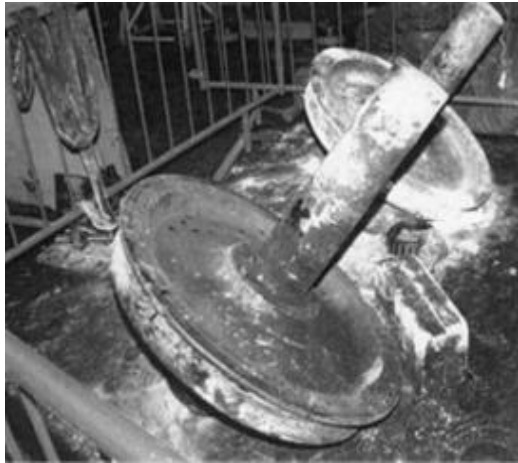
(a) Railway axle broken into two pieces from the freight wagon
