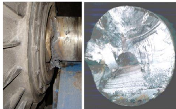
Figure 2.4: Fractures of traction shafts-axles in section 2 (Fig. 2.1).
