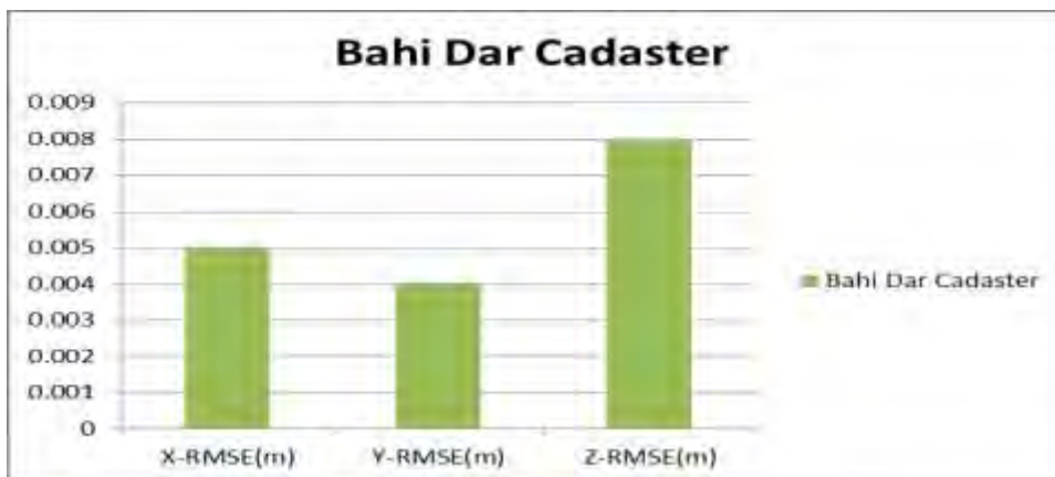
Figure 8: AT positional accuracy result of Bahir Dar cadaster.
