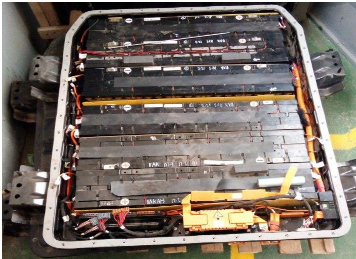
Figure 19. typical configuration of 150Ah Letin mengo (Anna 200) electric vehicle battery pack
