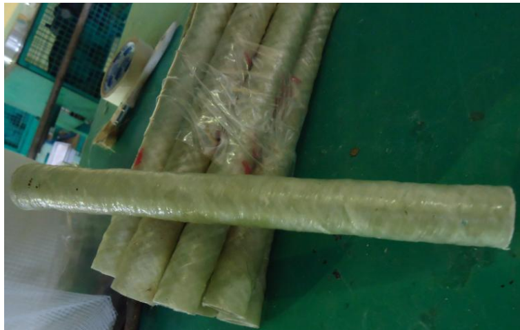
Figure 6-2: - Glass fiber-reinforced hollow circular shaft specimens
