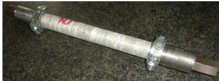
Figure 6-3: - Assembled specimen, end clamp and hose clip together
