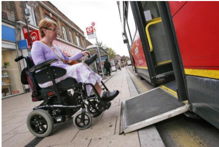
Figure 2-2 Sample low floored vehicle access
