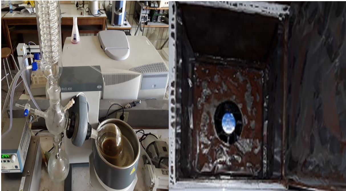
Fig. B - 5. Solvent recovery and drying of crude azadirachtin
