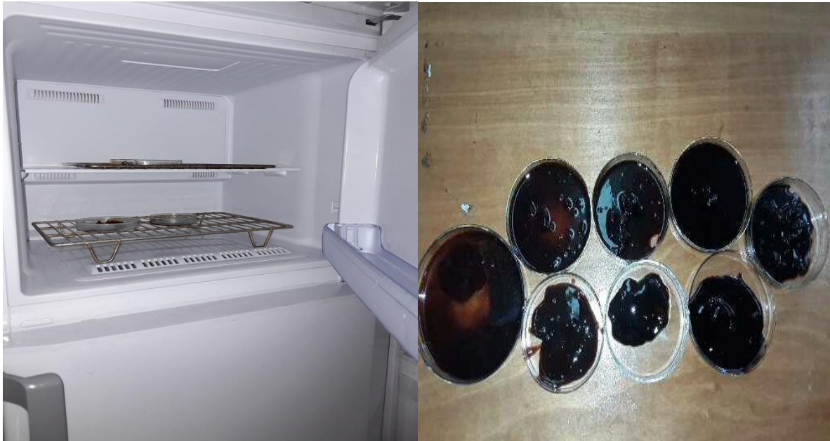
Fig. B – 7. Deep freeze-drying refrigerator and dried Azadirachtin
