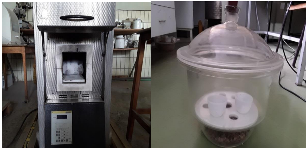
Figure 3-3. Muffle furnace and desiccator with crucible
