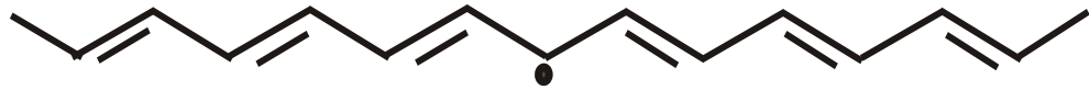
Figure 2.8: A domain wall ( soliton ) separating a trans-polyacetylene chain into domains similar to phase a and phase b in figure 2.7
